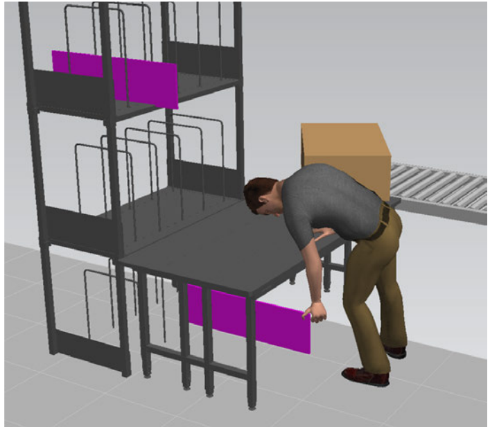
Figure 6: DHM reaching for boxes across 34in table (L) DHM bending and twisting to select box below pack station (R)
