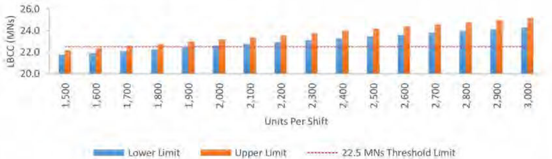
166 167 Figure 2: Low back cumulative compression values across multiple daily frequency exposures. The low back cumulative 168 compression values are inclusive of 90% of a mixed gender population by stature and weight. The proposed threshold limit for 169 low back cumulative compression is 22.5MNs represented by the dotted line on the graph.
